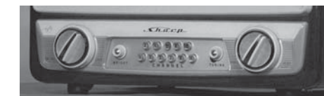
Push-button channel selector on the TB-50
