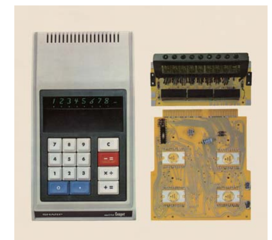
The QT-8D, the world's first LSI calculator (left) and its substrate fitted with MOS LSI
