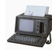
Word processor equipped with an AI dictionary for converting entire typed clauses into kanji
