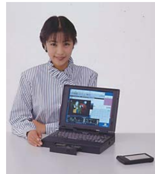
The AV1/590CD notebook PC used an 11.3-inch SVGA (800 × 600-dot) color TFT LCD that was 40% brighter than previous Sharp LCDs
