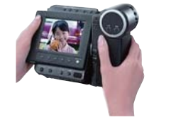
LCD ViewCam, which allowed users to shoot video while watching an LCD viewfinder and enabled instant playback of just-taken footage
