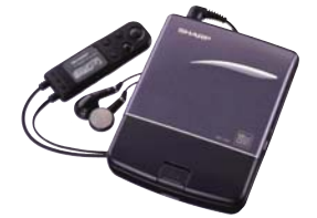
The MD-S10 MD player came with a remote control equipped with an LCD
