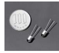
Double LED capable of simultaneously emitting visible light and near-infrared light
