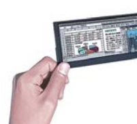
High-reflective Super Mobile LCD for the outdoor display of bright color images without the need for a backlight
