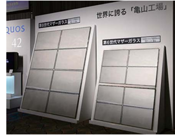
Sixth-generation glass substrate (right) from Plant No. 1 and eighth-generation glass substrate (left) from Plant No. 2, which started operations in August 2006
