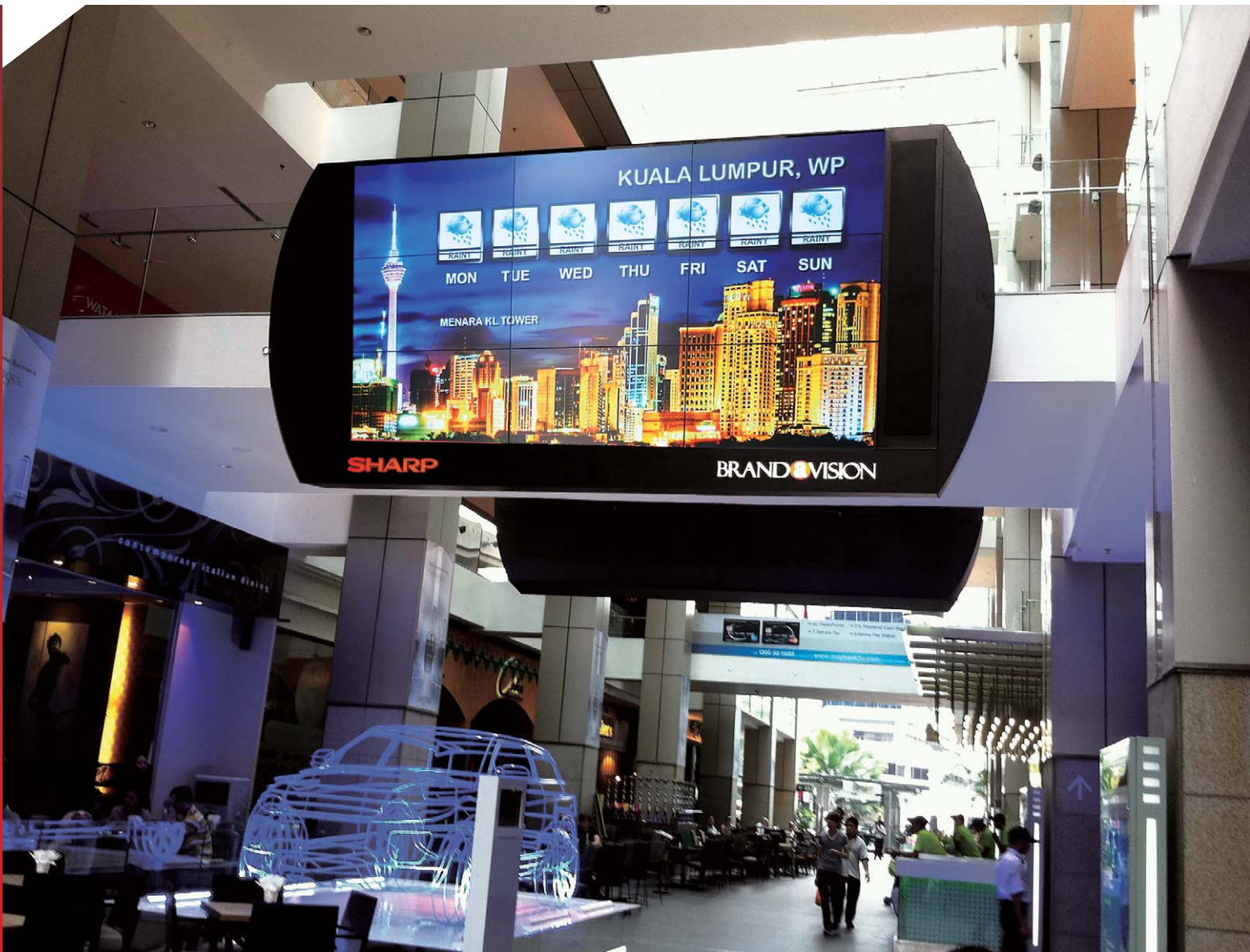
Multi-screen display systems at a shopping mall in Malaysia (9 large-size LCD monitors are used for each display system installed on both sides of a connecting corridor)
