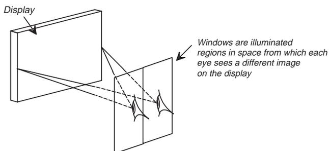
Fig. 1 Generation of windows in autostereoscopic displays.
