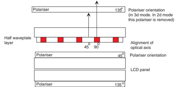
Fig. 6 2d/3d display configuration.
