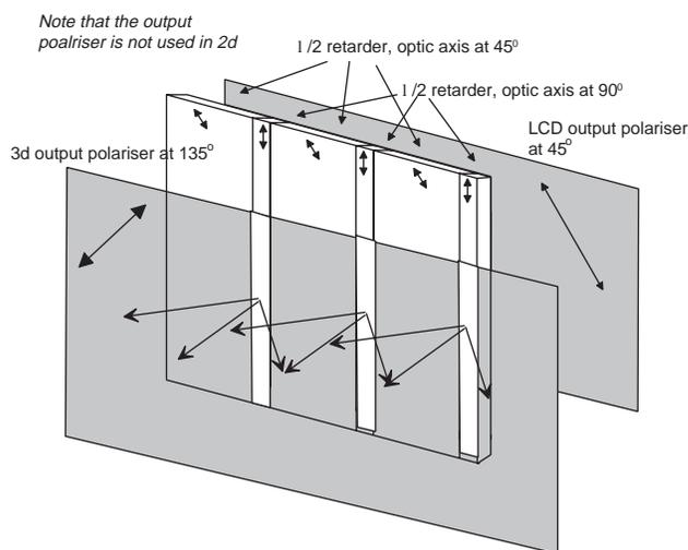
Fig. 3 Retarder Parallax barrier configuration.
