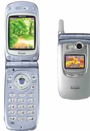
Fig. 1 SH251iS Mobile phone with 2D/3D display.
