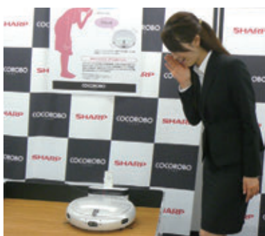
The voice recognition function makes it possible for the robot to respond to your commands
