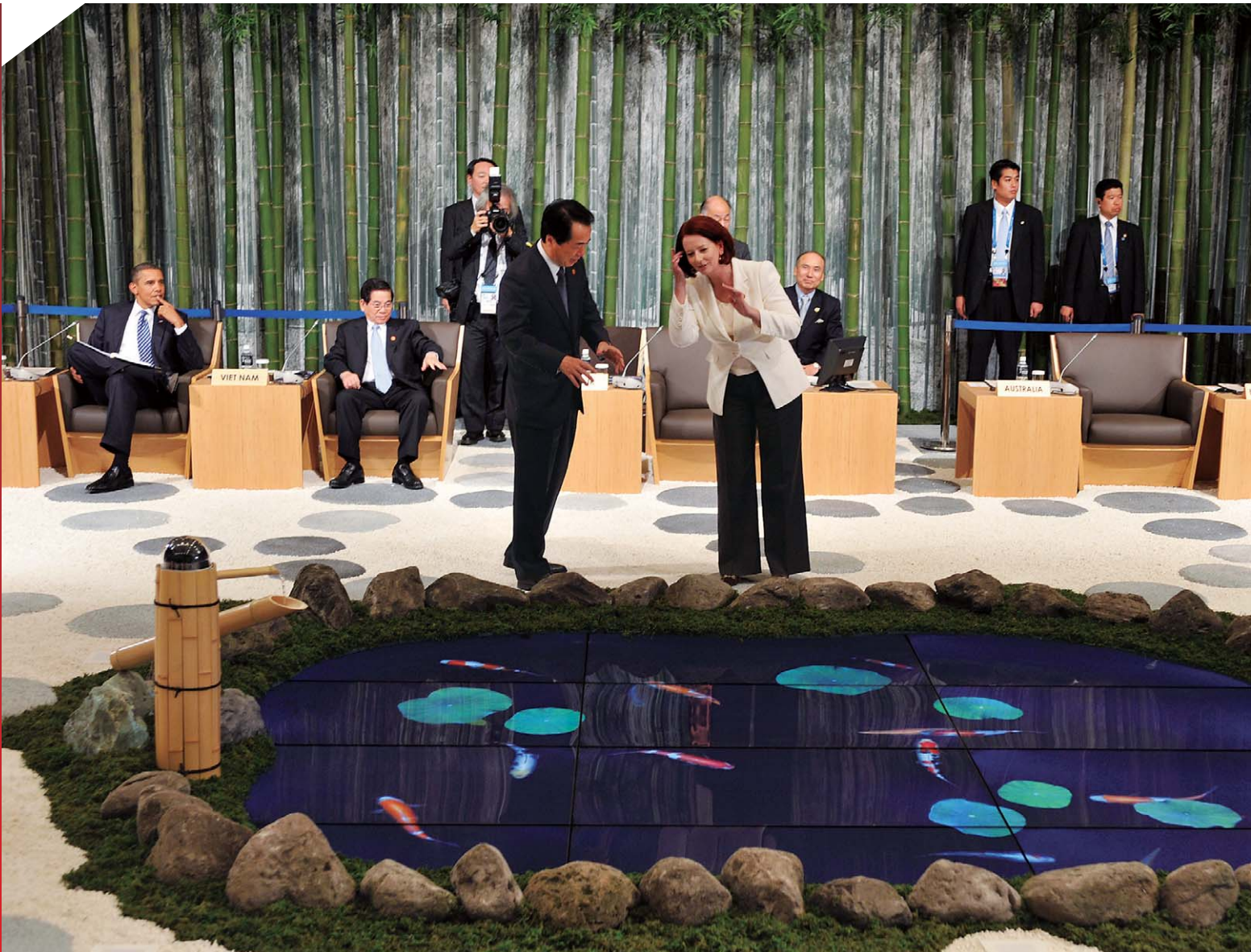
Multi-screen display system used in the venue for the APEC Japan 2010 Economic Leaders' Meeting (12 large-size LCD monitors used to reproduce a pond)
