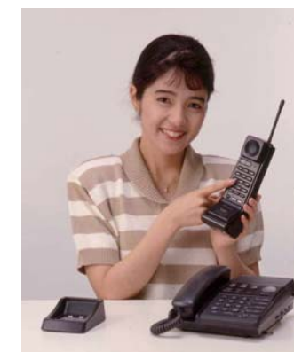
The CJ-A300 could control answering machine functions via the handset and make calls from the base unit, which was not possible on previous models
