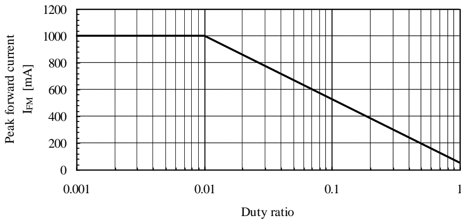
Fig.3 Peak forward current vs. duty ratio
