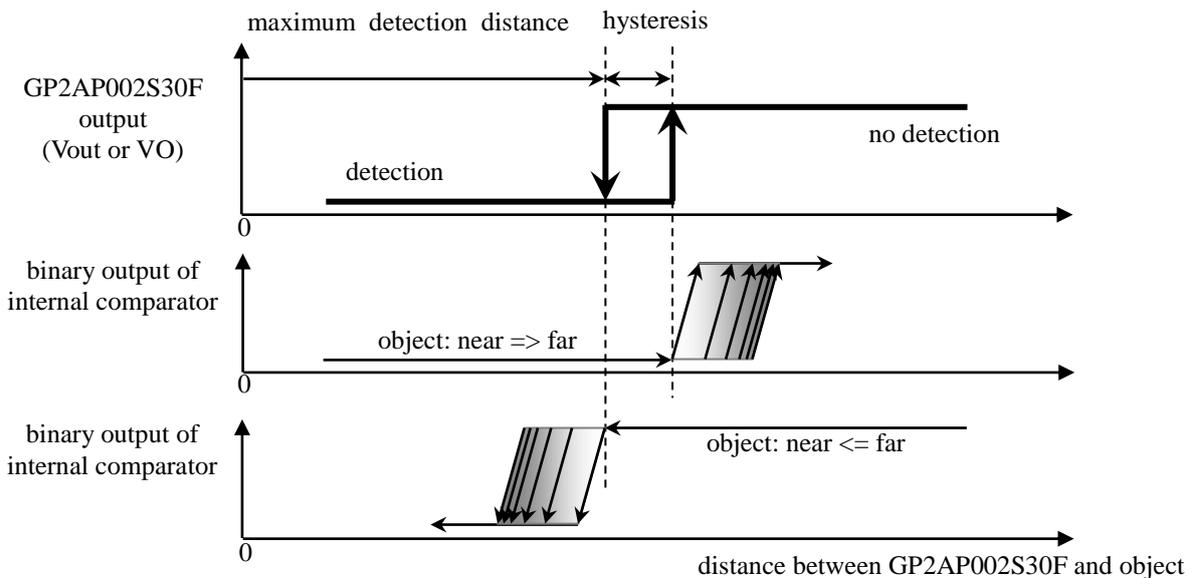
Note that the detection distance can be controlled by changing LED current limiting resistor, too.
