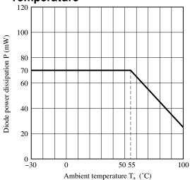
Fig.4 Total Power Dissipation vs. Ambient Temperature
