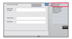
Tap [Direct Input of Folder Path] in step 3 of "Printing a file in the network folder you have configured in the machine's settings (page 3-78)".
