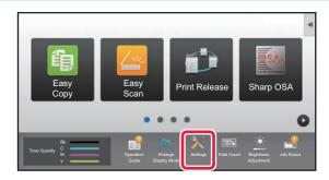
Make sure that the Data Notification indicator is blinking, and tap the [Settings] key in the home screen.
