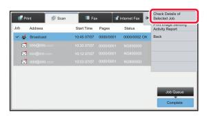
After tapping the key of the completed broadcast transmission, tap [Check Details of Selected Job] on the action panel.
