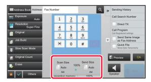
In the above screen, the scan size (the placed original) is A4 (8-1/2" x 11") and the send size is auto. For example, if the scan size is A4 (8-1/2" x 11") and the send size is B5 (5-1/2" x 8-1/2"), the image will be reduced before transmission.
