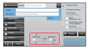
In the above screen, the scan size (the placed original) is A4 (8-1/2"  $\times$  11") and the send size is auto. For example, if the scan size is A4 (8-1/2"  $\times$  11") and the send size is B5 (5-1/2"  $\times$  8-1/2"), the image will be reduced before transmission.
