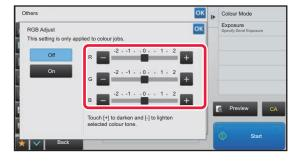
Tap - + of the colour you want to adjust or slide the slider to adjust the colouring.
