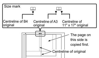
Align the centre of the original with the appropriate size mark  $lack \Psi$  .
