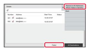
After tapping the [Failed] tab, tap [Resend to All Addresses Which Failed in Sending] on the action panel to resend the image.
