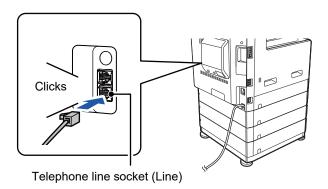
In some countries, an adaptor is required to connect the telephone line cable to the wall telephone socket, as shown in the illustration.
