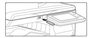
Check the [Sending data has been completed.] message, and remove the USB memory device from the machine.
