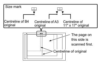
Align the centre of the original with the appropriate size mark
