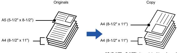
A5  $(5-1/2" \times 8-1/2")$  size original is enlarged to A4  $(8-1/2" \times 11")$  size for printing.
