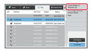
After tapping the key of the completed broadcast transmission, tap [Check Details of Selected Job] on the action panel.
