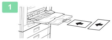
Place the transparency film face down in the bypass tray, and load transparency film sheets.
