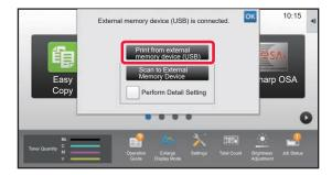
When the screen for selecting the action appears, tap [Print from external memory device (USB)].
