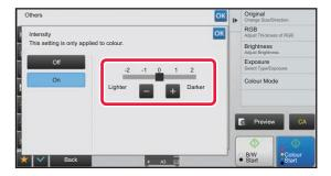
Tap the key or slide the slider to adjust the intensity.
