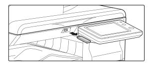
Remove the USB memory device from the machine.
