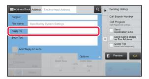
To change the reply address, tap the [Reply-To] entry box.
