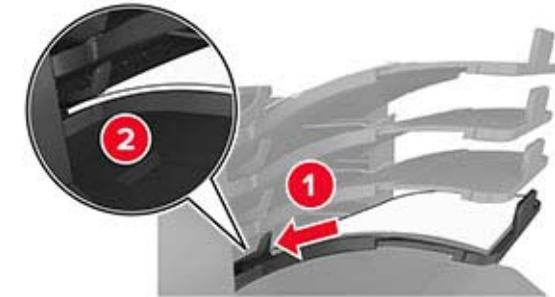
**Note:** If the paper is not under the bin arm, then a jam occurs due to an overfilled bin.
